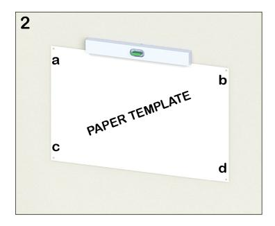
**2.** In order to facilitate installation we have included a paper template to drill the holes in the wall.
